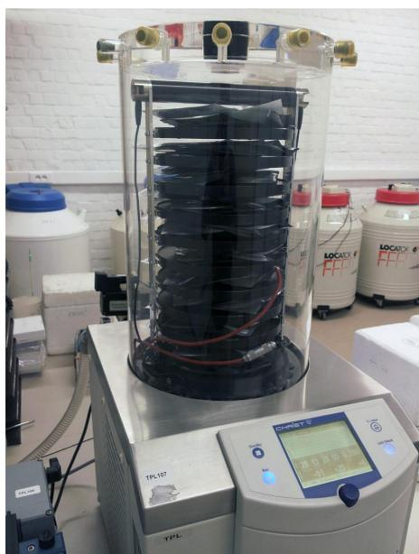
Freeze-drying device for leaf samples
